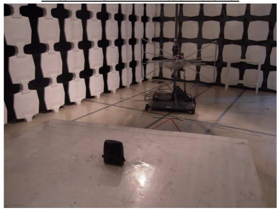
MEASUREMENT OF CONDUCTED EMISSION TEST SET UP
