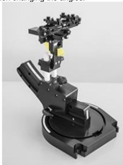
Device holder supplied by SPEAG
