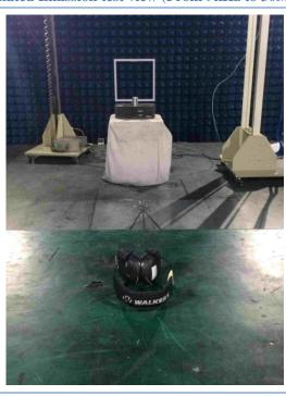
Radiated Emission test view (From 30MHz to 1GHz)
