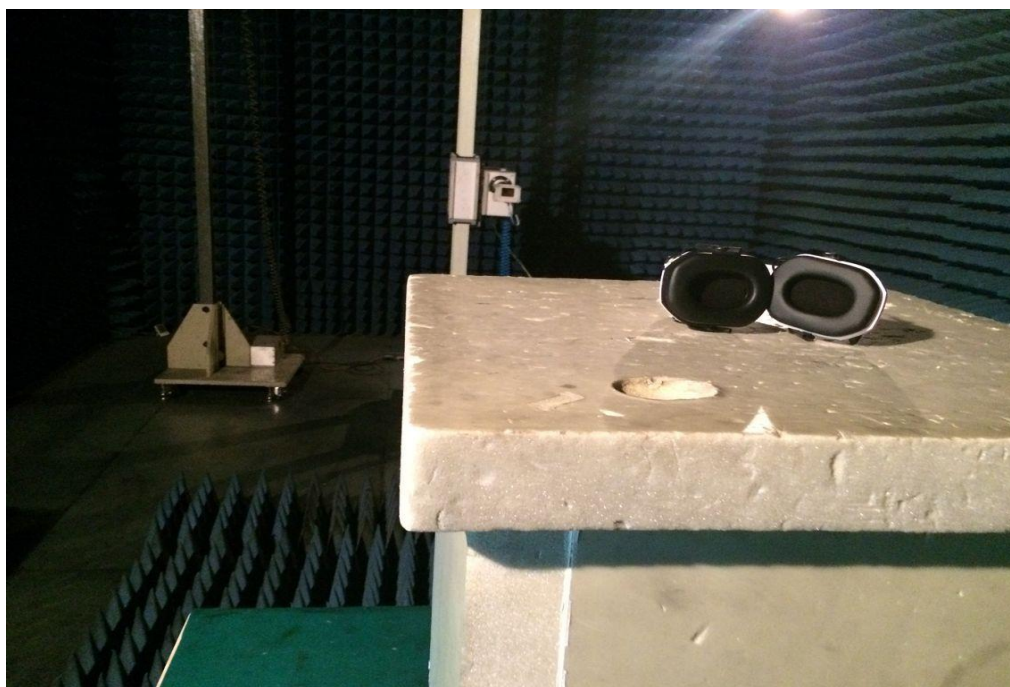
Radiated Emission test view (18GHz to 26.5GHz)
