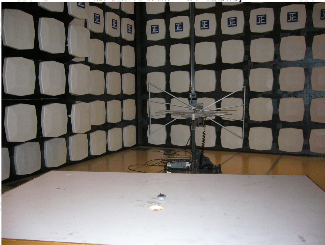
Measurement of Radiated Emission Test Set Up
