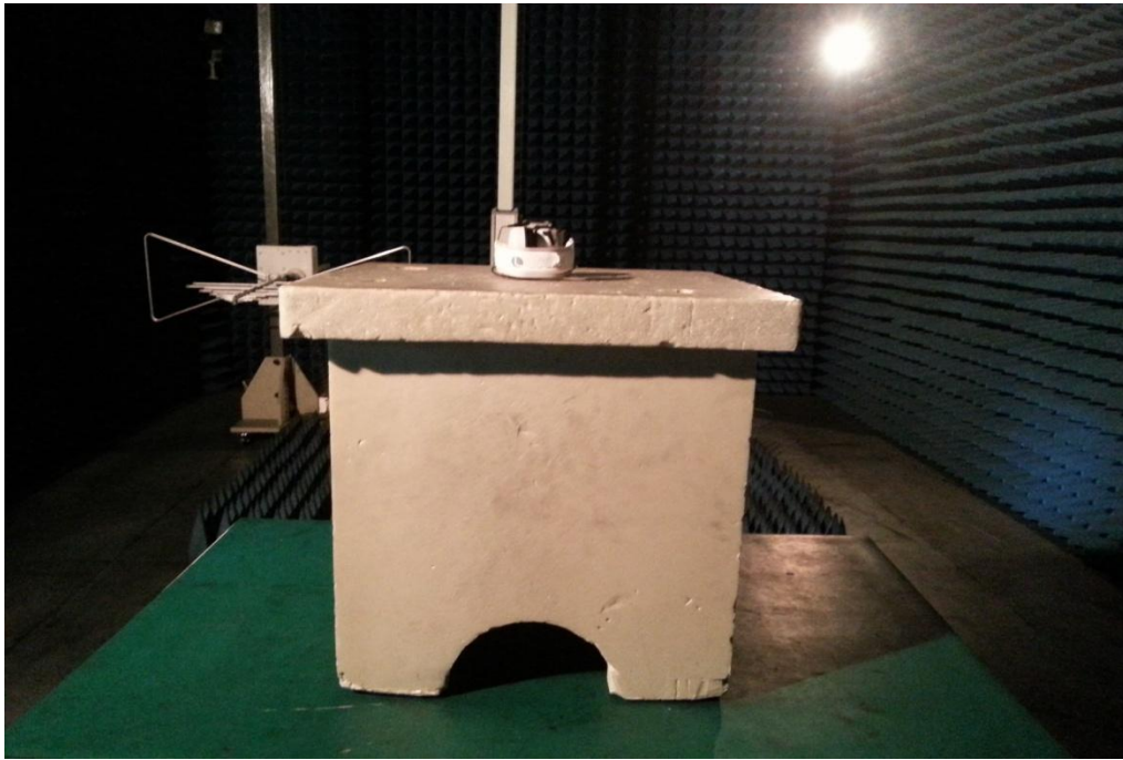
Radiated Emission test view (1GHz to 18GHz)
