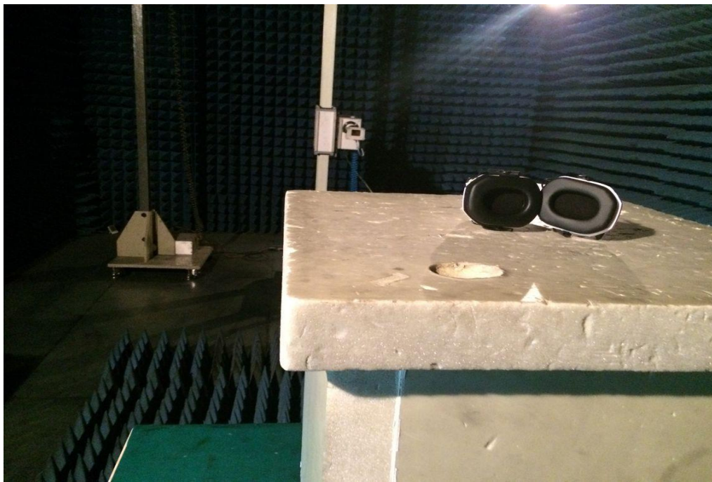
Radiated Emission test view (18GHz to 26.5GHz)
