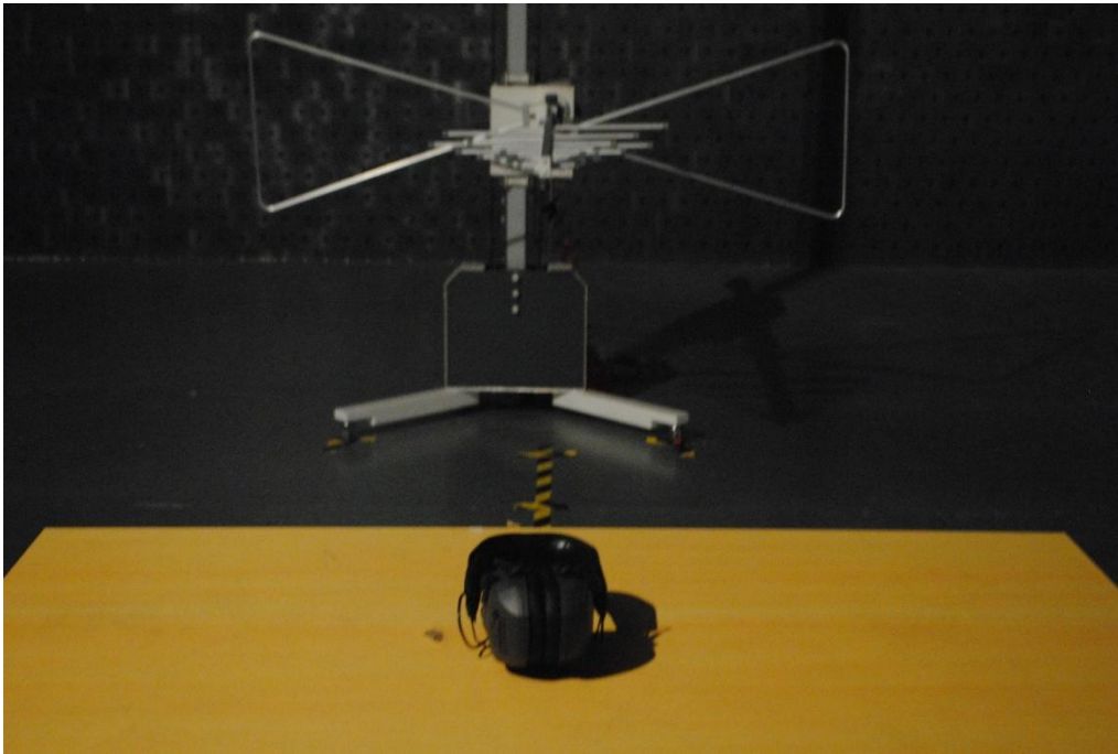
Radiated Emission test view (Frequency above 1GHz)
