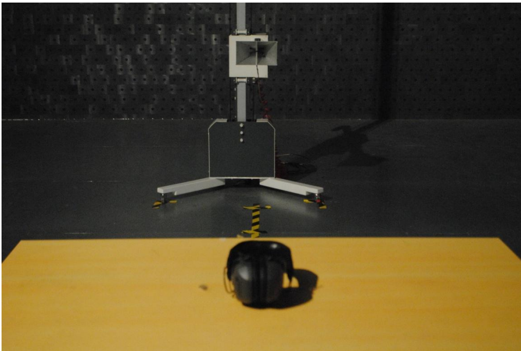
Radiated Emission test view (Frequency above 1GHz)
