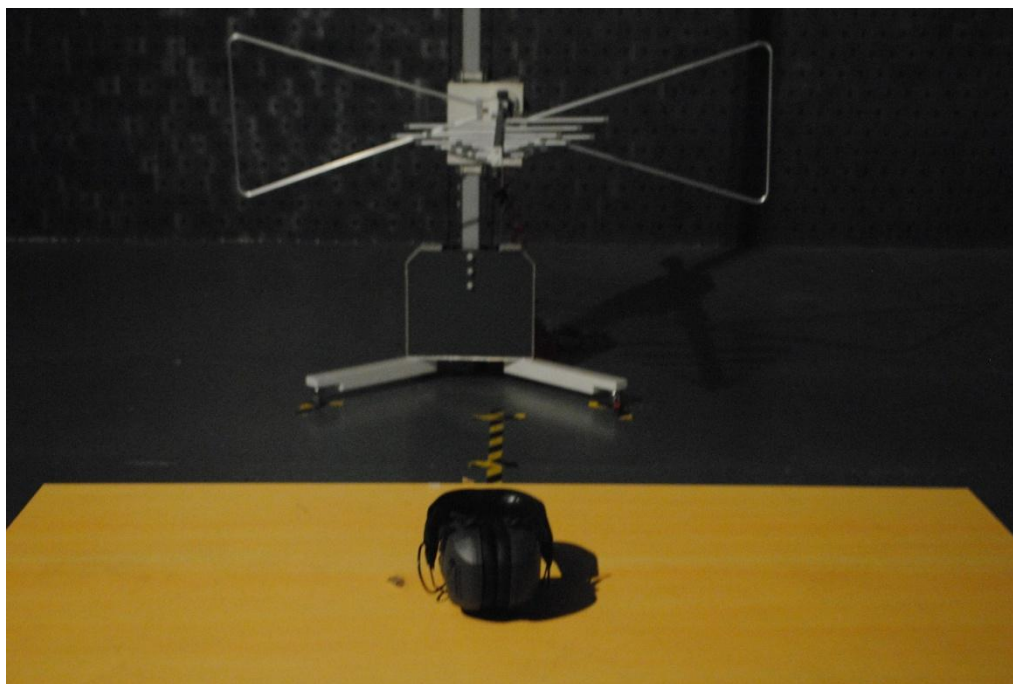
Radiated Emission test view (Frequency above 1GHz)
