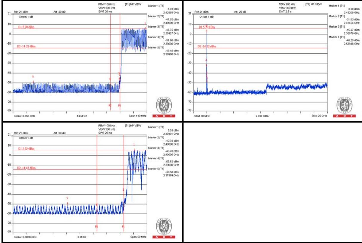
**Hopping enabled\_ High Channel**
