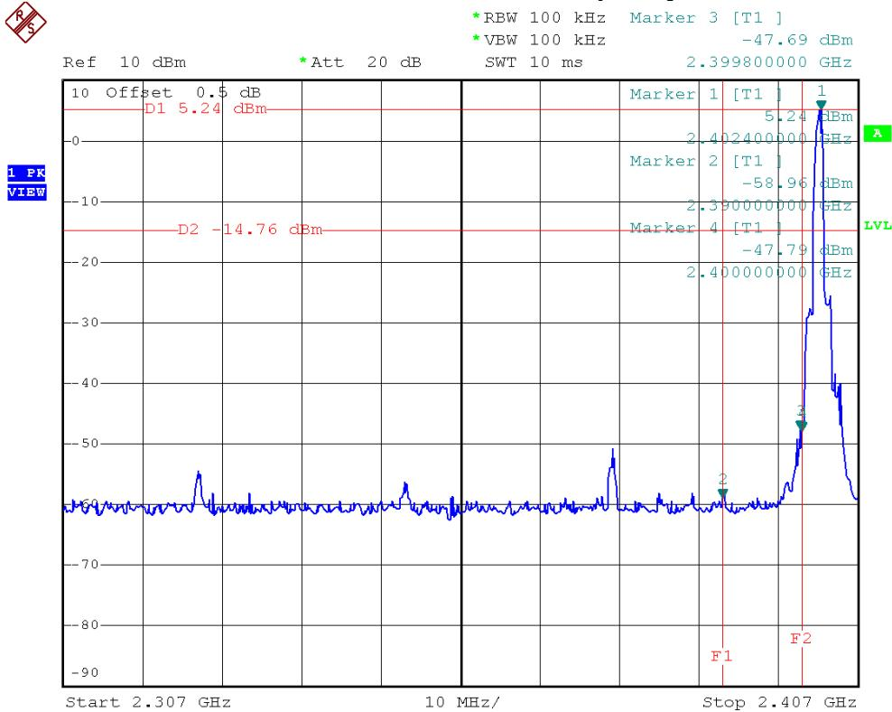
**Bluetooth/3 Mbps/The max. radio frequency power in any 100 kHz bandwidth within the frequency band**
