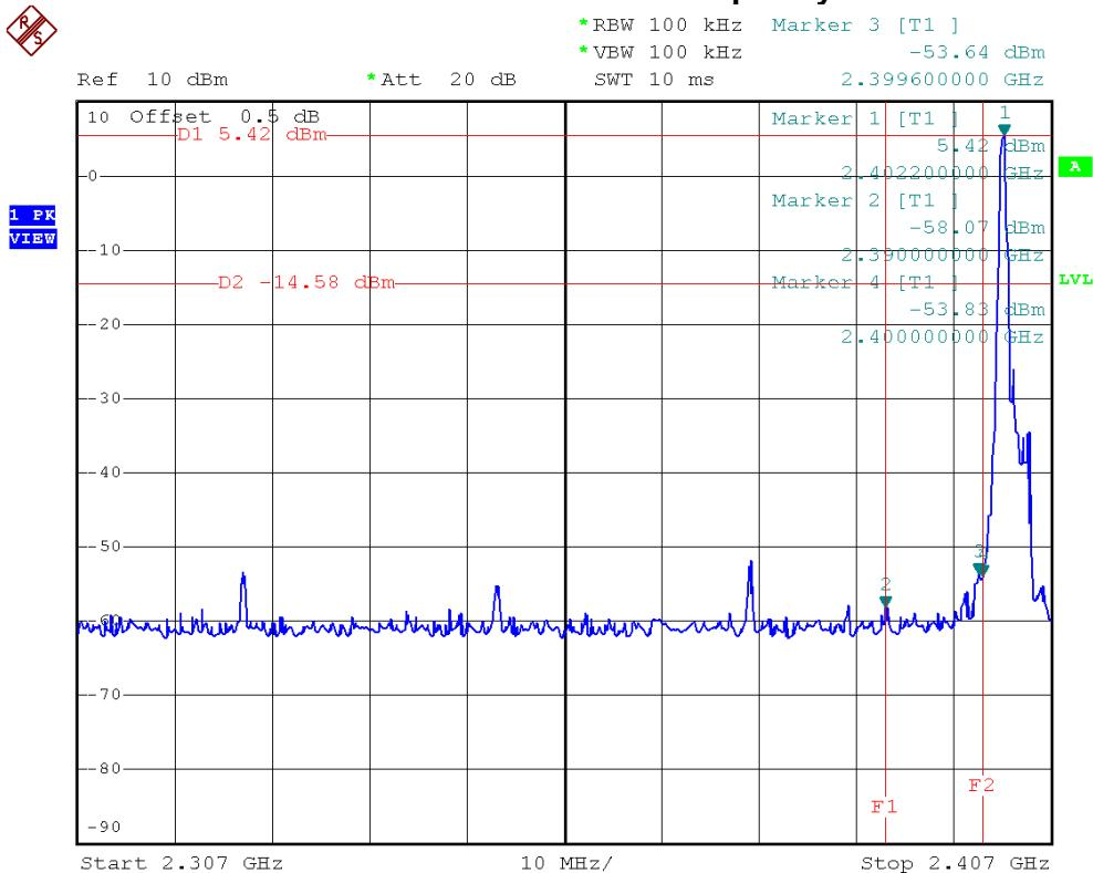
**Bluetooth/1 Mbps/The max. radio frequency power in any 100 kHz bandwidth within the frequency band**
