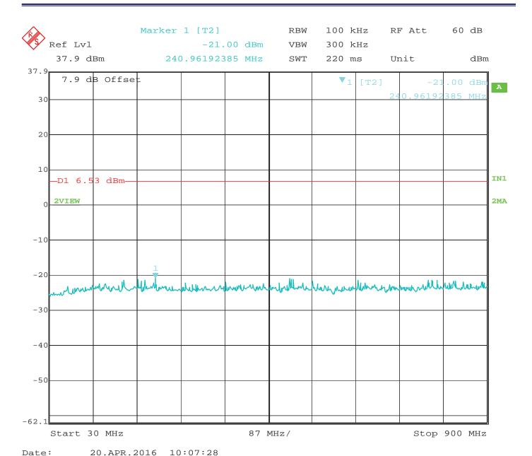
RF Antenna Conducted - Middle Channel - 30 MHz to 900 MHz - Configuration #2 - Port #1 Worst Case
