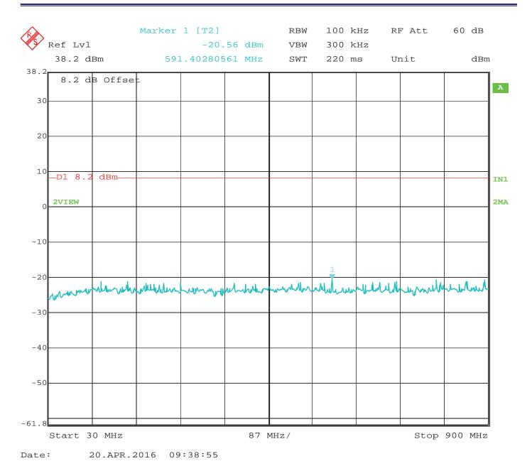
RF Antenna Conducted – High Channel – 30 MHz to 900 MHz – Configuration #1 – Port #4 Worst Case
