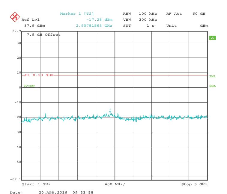
RF Antenna Conducted - Middle Channel - 1 GHz to 5 GHz - Configuration #1 - Port #4 Worst Case
