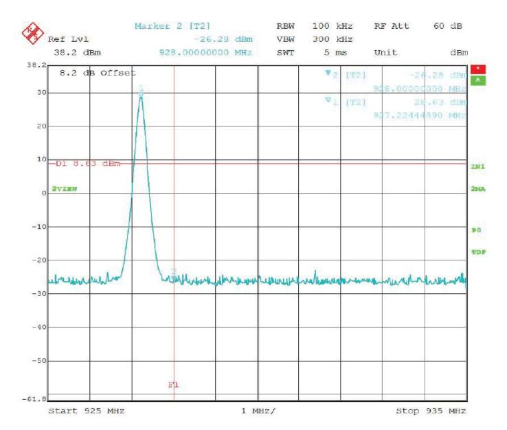
Band Edge - High Channel - Fixed Frequency Mode - Configuration #1 - Port #4 Worst Case
