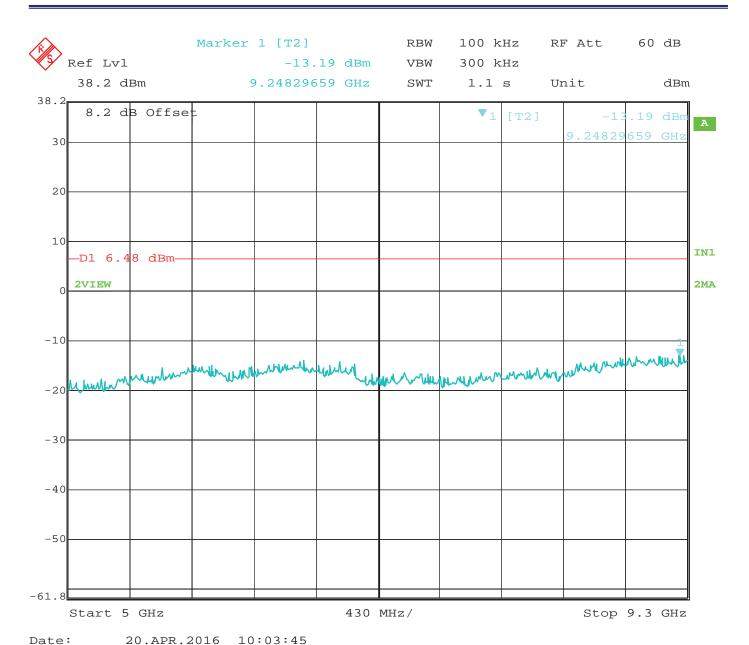
RF Antenna Conducted - High Channel - 5 GHz to 9.3 GHz - Configuration #2 - Port #1 Worst Case
