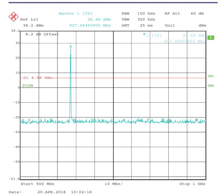
RF Antenna Conducted – High Channel – 900 MHz to 1 GHz – Configuration #2 – Port #1 Worst Case
