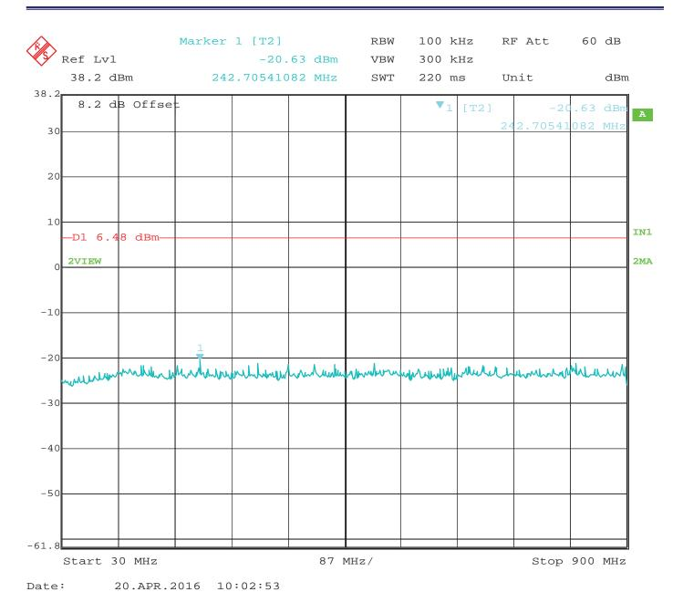
RF Antenna Conducted – High Channel – 30 MHz to 900 MHz – Configuration #2 – Port #1 Worst Case
