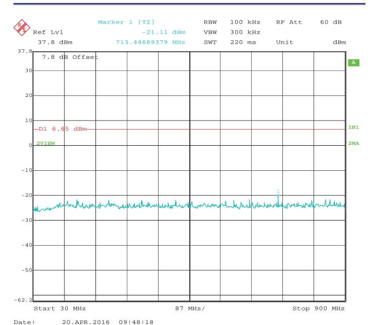
RF Antenna Conducted – Low Channel – 30 MHz to 900 MHz – Configuration #2 – Port #1 Worst Case
