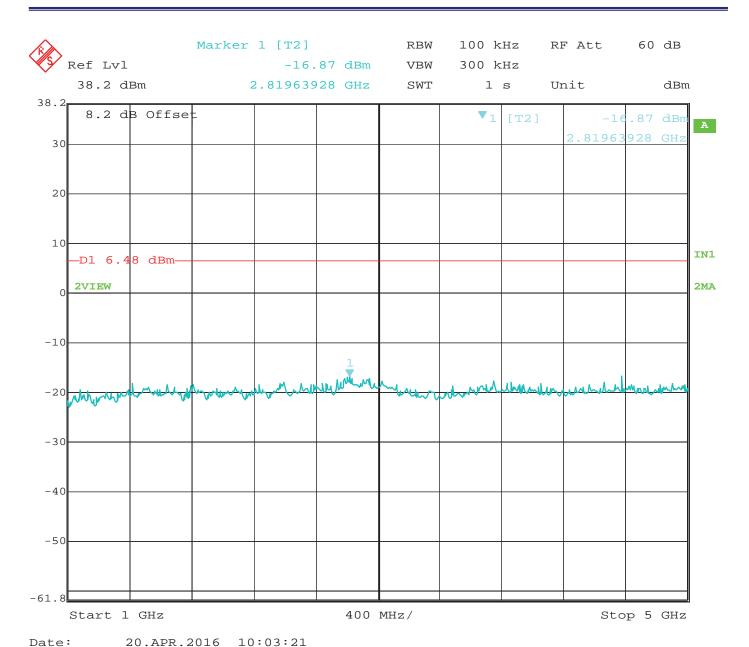
RF Antenna Conducted - High Channel - 1 GHz to 5 GHz - Configuration #2 - Port #1 Worst Case
