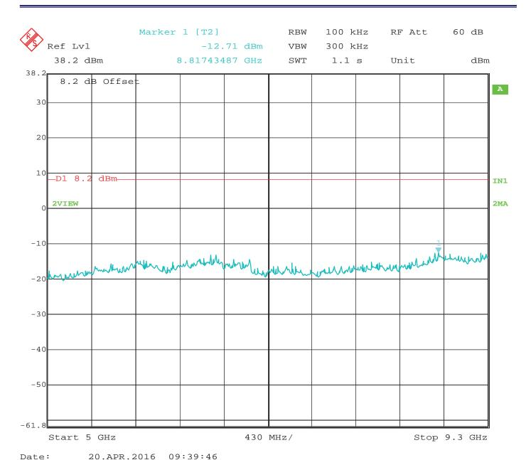
RF Antenna Conducted – High Channel – 5 GHz to 9.3 GHz – Configuration #1 – Port #4 Worst Case
