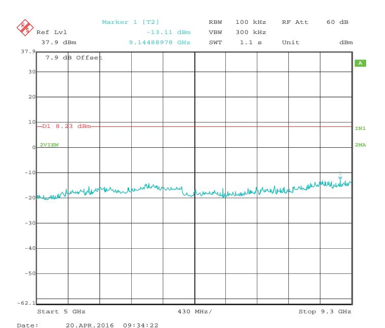
RF Antenna Conducted - Middle Channel - 5 GHz to 9.3 GHz - Configuration #1 - Port #4 Worst Case
