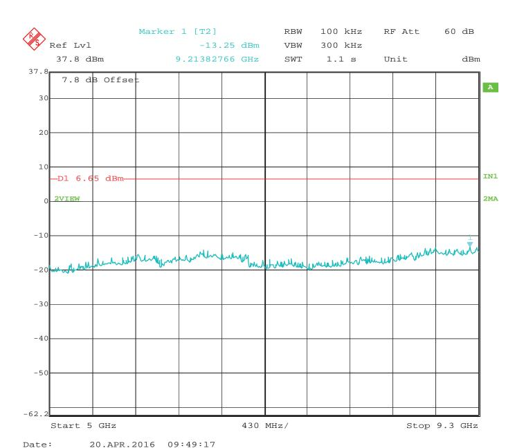
RF Antenna Conducted - Low Channel - 5 GHz to 9.3 GHz - Configuration #2 - Port #1 Worst Case
