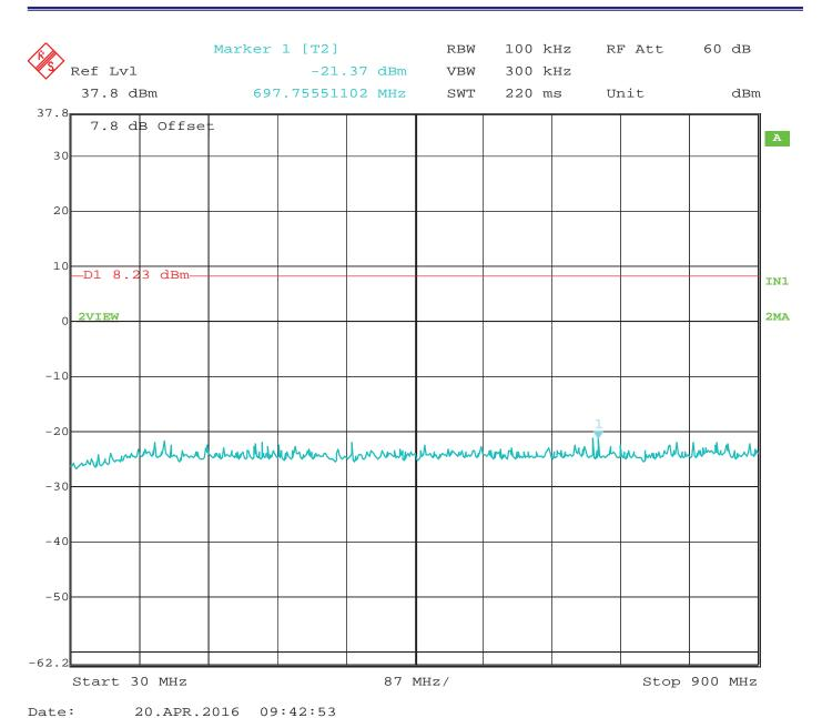
RF Antenna Conducted - Low Channel - 30 MHz to 900 MHz - Configuration #1 - Port #4 Worst Case
