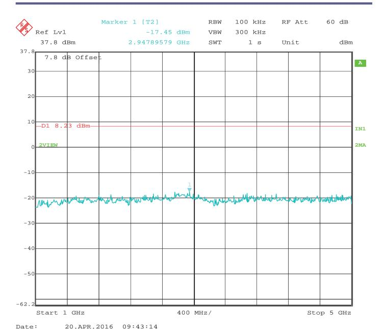
RF Antenna Conducted - Low Channel - 1 GHz to 5 GHz - Configuration #1 - Port #4 Worst Case
