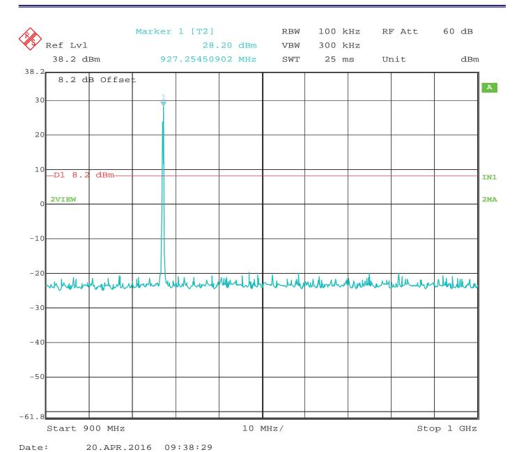
RF Antenna Conducted – High Channel – 900 MHz to 1 GHz – Configuration #1 – Port #4 Worst Case
