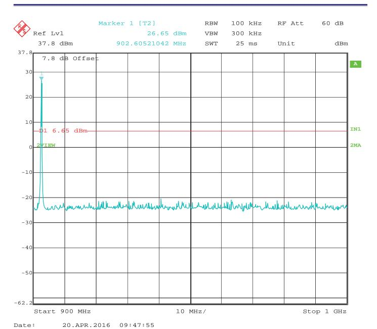
RF Antenna Conducted - Low Channel - 900 MHz to 1 GHz - Configuration #2 - Port #1 Worst Case
