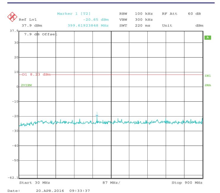
RF Antenna Conducted – Middle Channel – 30 MHz to 900 MHz – Configuration #1 – Port #4 Worst Case
