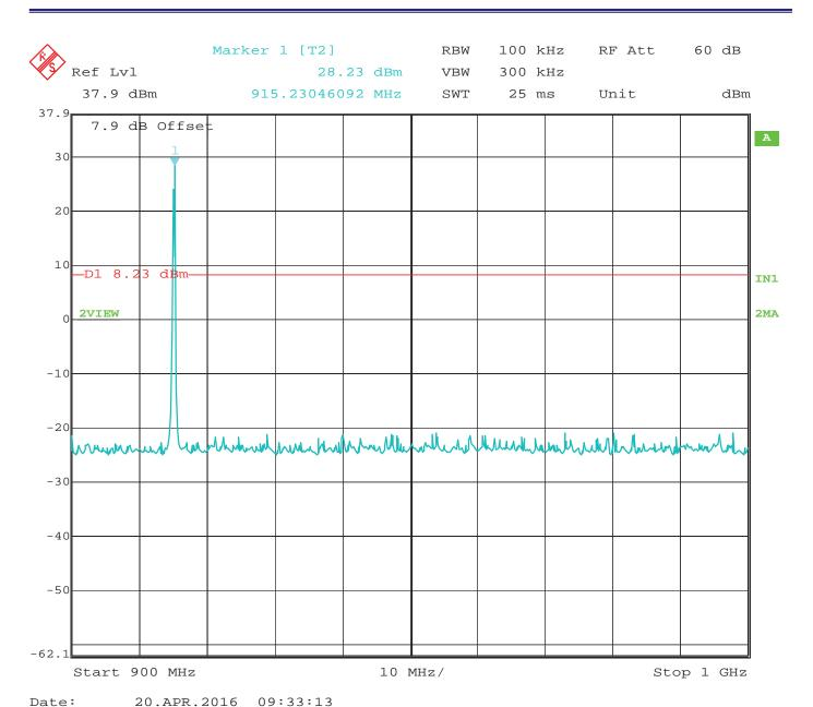
RF Antenna Conducted - Middle Channel - 900 MHz to 1 GHz - Configuration #1 - Port #4 Worst Case
