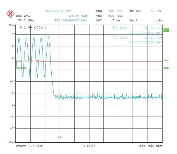
Band Edge - High Channel - Frequency Hopping Mode - Configuration #2 - Port #1 Worst Case
