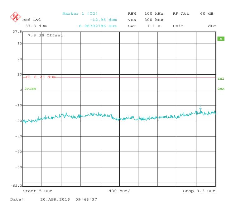
RF Antenna Conducted - Low Channel - 5 GHz to 9.3 GHz - Configuration #1 - Port #4 Worst Case
