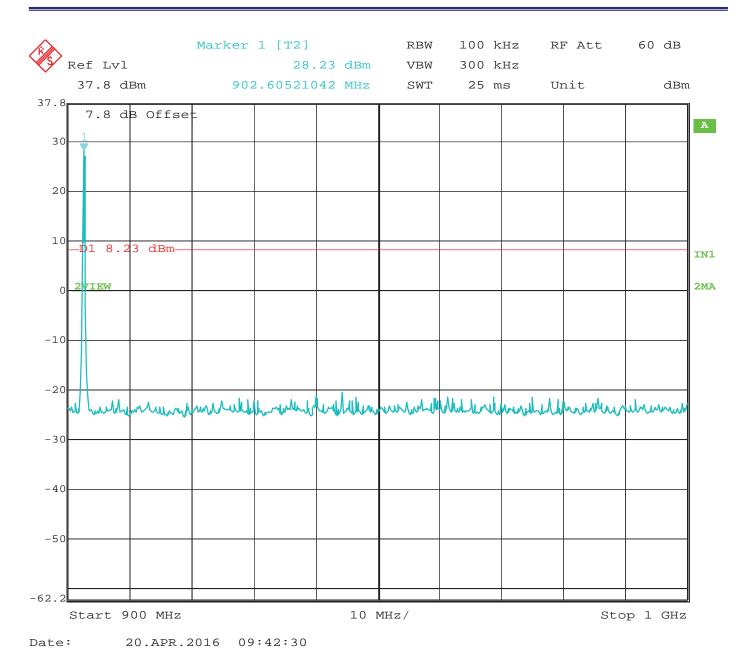
RF Antenna Conducted - Low Channel - 900 MHz to 1 GHz - Configuration #1 - Port #4 Worst Case
