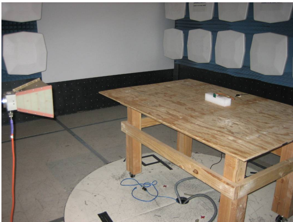
Radiated Emission Setup View (> 1GHz)
