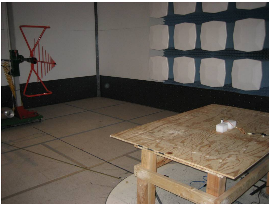
Radiated Emission Setup View (< 1GHz)
