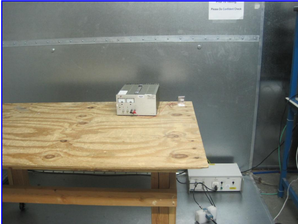
Conducted Emission Test Setup – Front View
