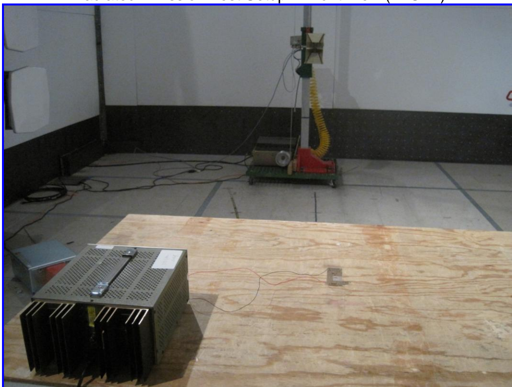
Radiated Emission Test Setup – Rear View (>1GHz)
