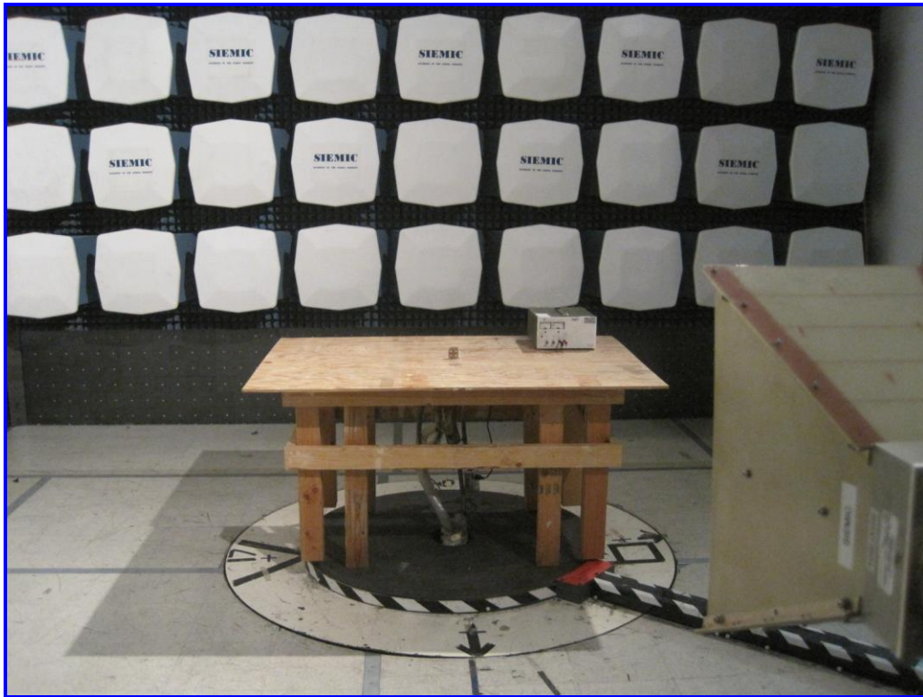
Radiated Emission Test Setup – Front View (>1GHz)
