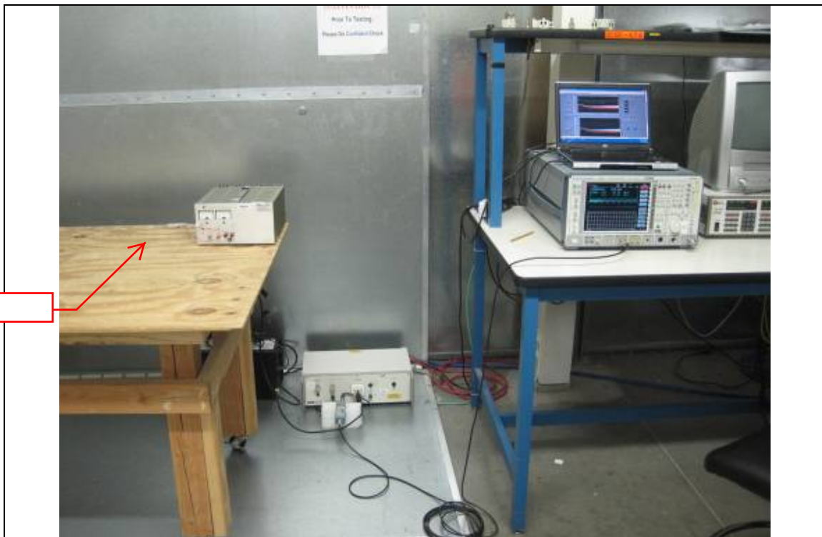
Conducted Emission Test Setup – Front View
