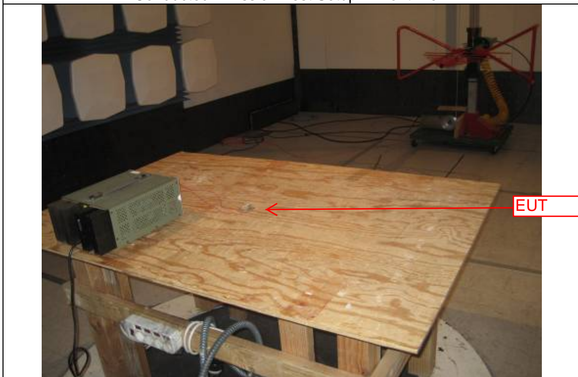
Radiated Emission Test Setup – (Below 1GHz) Worst orientation
