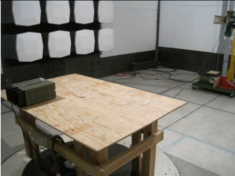
Radiated Emission Test Setup – (Above 1GHz) Worst orientation
