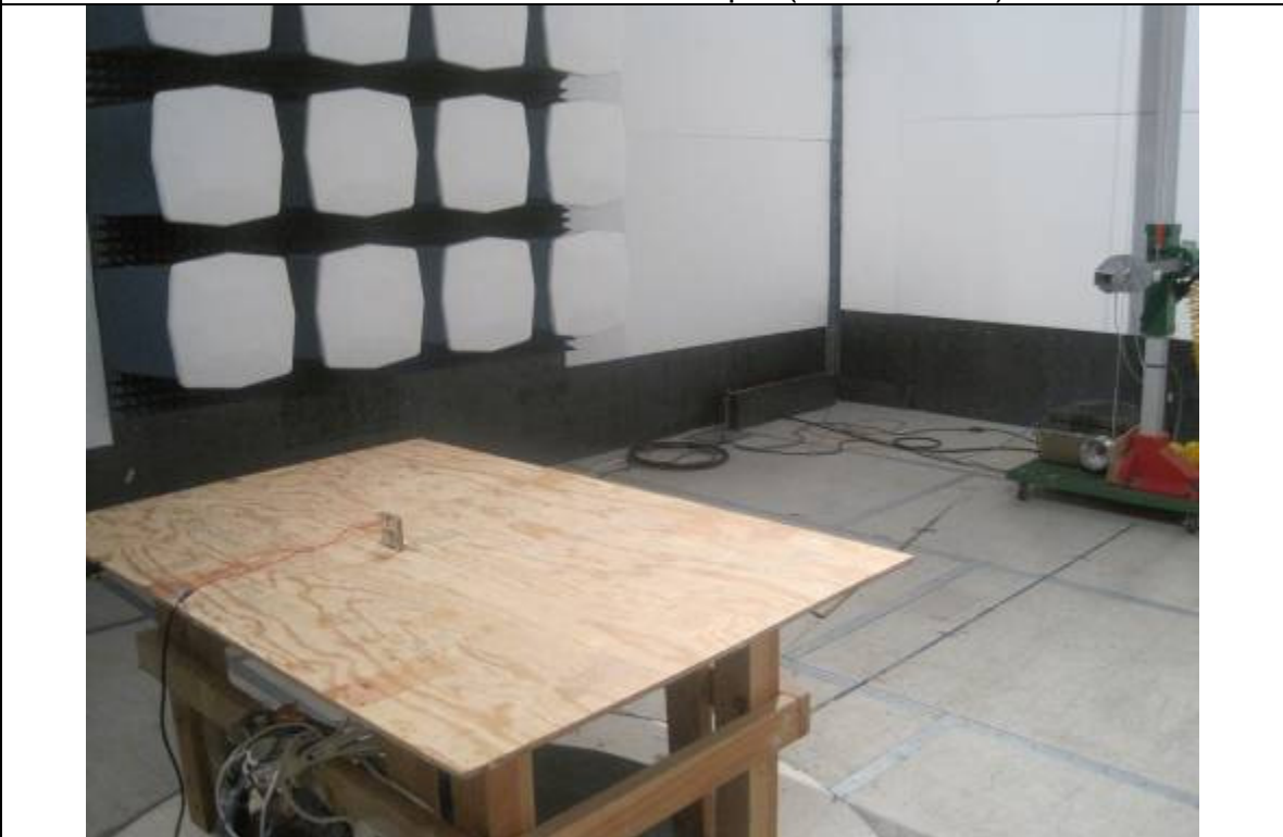
Radiated Emission Test Setup –(Above 18GHz)
