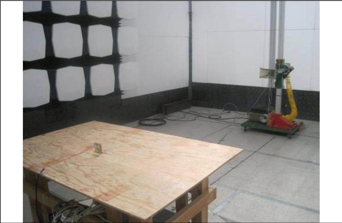
Radiated Emission Test Setup – (Above 1GHz)
