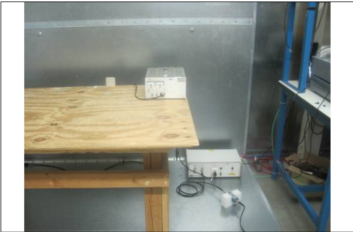
Conducted Emission Test Setup – Front View
