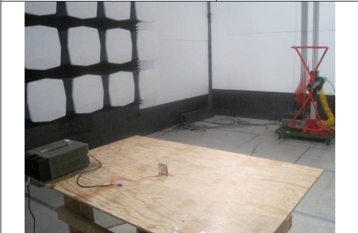
Radiated Emission Test Setup – (Below 1GHz)
