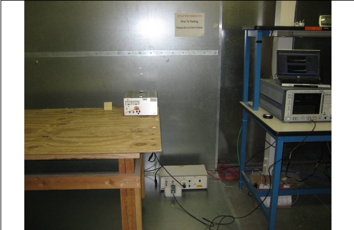
Conducted Emission Test Setup – Front View
