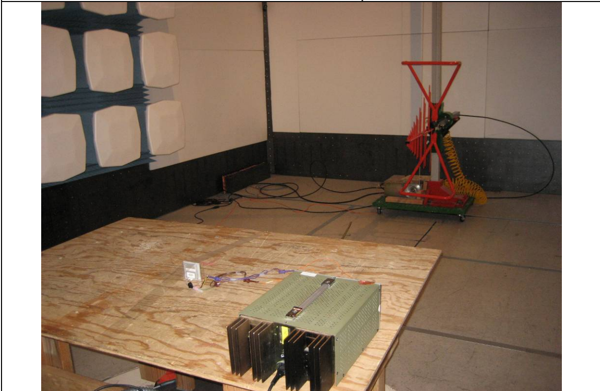
Radiated Emission Test Setup – (Below 1GHz)
