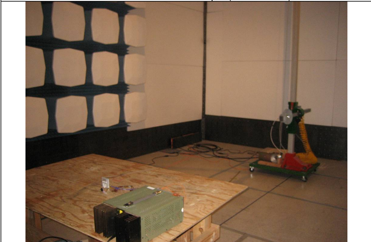
Radiated Emission Test Setup –(Above 18GHz)
