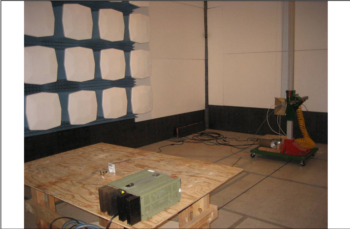
Radiated Emission Test Setup – (Above 1GHz)
