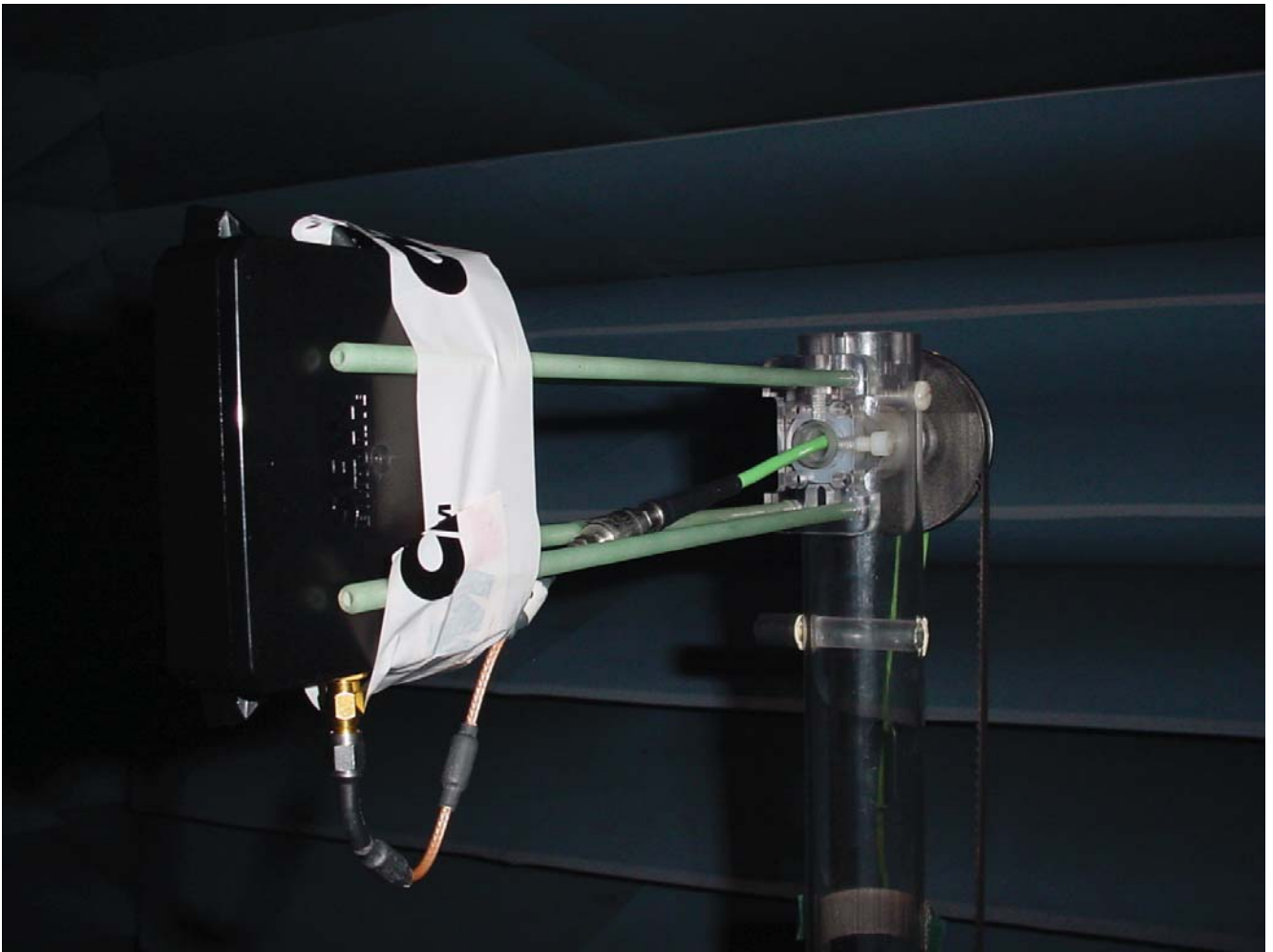
Setup A, C, E, G: azimuth angle = 0^\circ (antenna under test vertically oriented) Photo shows reference position at roll axis = 0^\circ (elevation)
