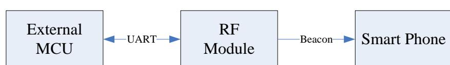
1. Send Command 'R' to send live measured data from external through Beacon.
