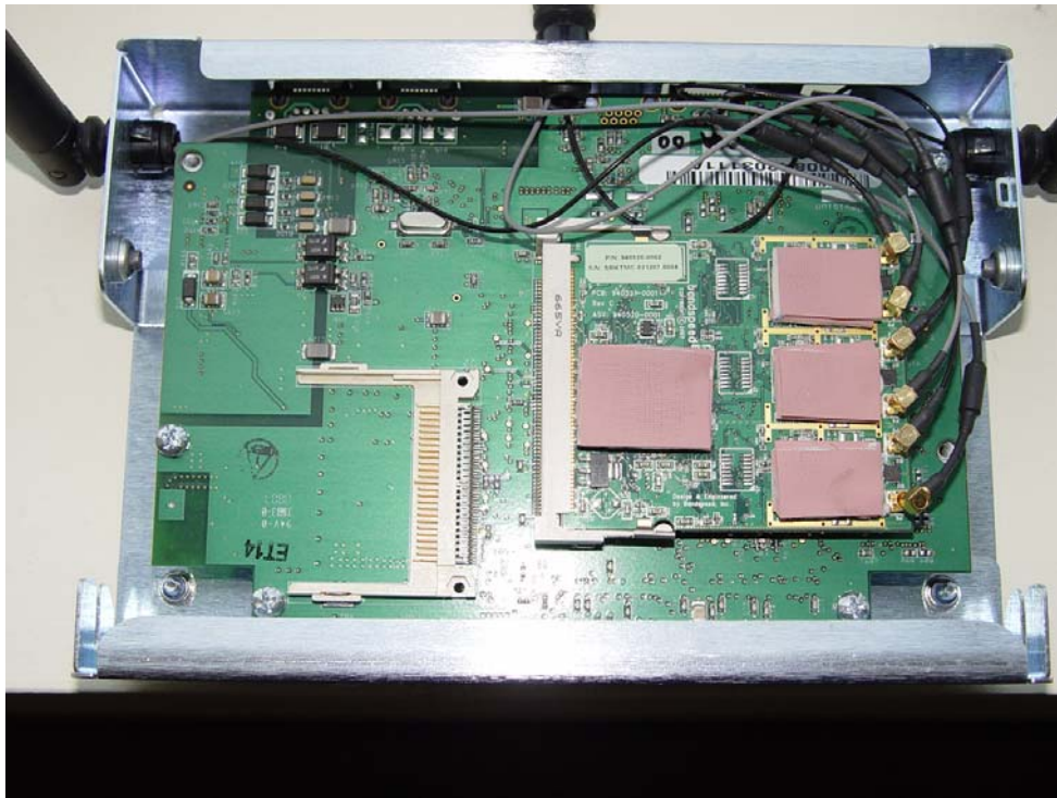
Internal View of Access Point
