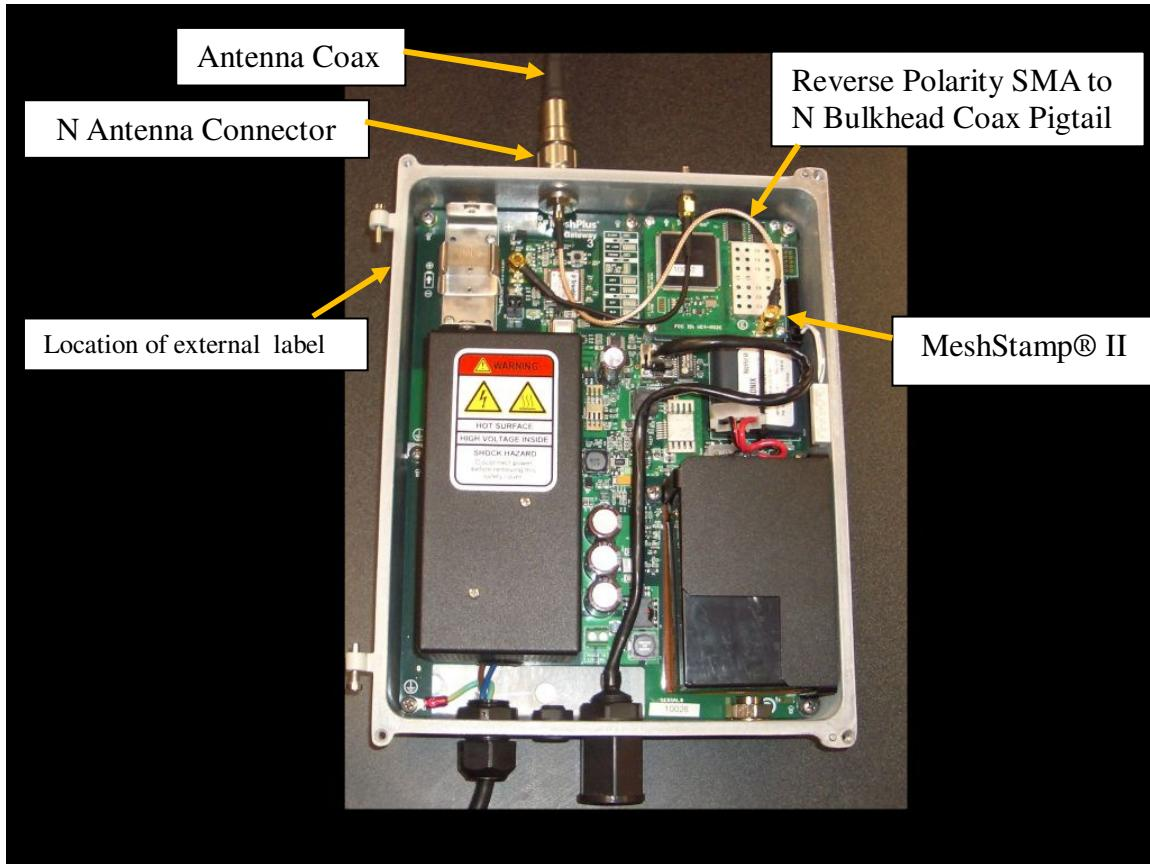
The MeshStamp II is plugged into the Ethernet Gateway motherboard at the top right of the enclosure. An N bulkhead antenna connector is attached to the top of the enclosure with a coax pigtail which connects to the reverse polarity SMA connector of the MeshStamp II. The remote mounted 8 dBi vertical antenna (the antenna used during compliance testing) is connected to the enclosure bulkhead antenna connector by coax cable.
