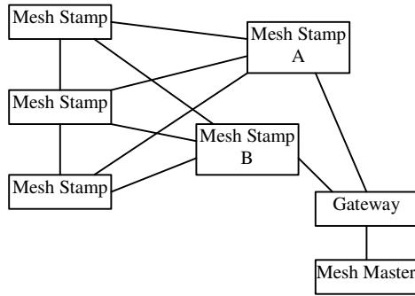
Build a mesh configuration where the traffic from three nodes traverses two others. Verify that data is being received from all five Mesh Stamps. Then turn the power off on Mesh Stamp A. Verify that data is being received from the remaining four Mesh Stamps.
