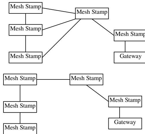
mesh, the Mesh Stamps must be separated so that they are not all communicating directly with the Gateway.
