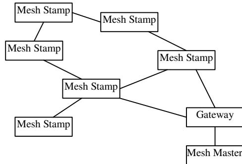
The MeshPlus® is a network of MeshStamps® where a MeshStamp® is typically a network data collection point associated with some external equipment which is monitored or controlled. In addition to local data collection, each MeshStamp® has the capability to receive and relay information from its neighbor MeshStamps® as well as transmit its own information.
