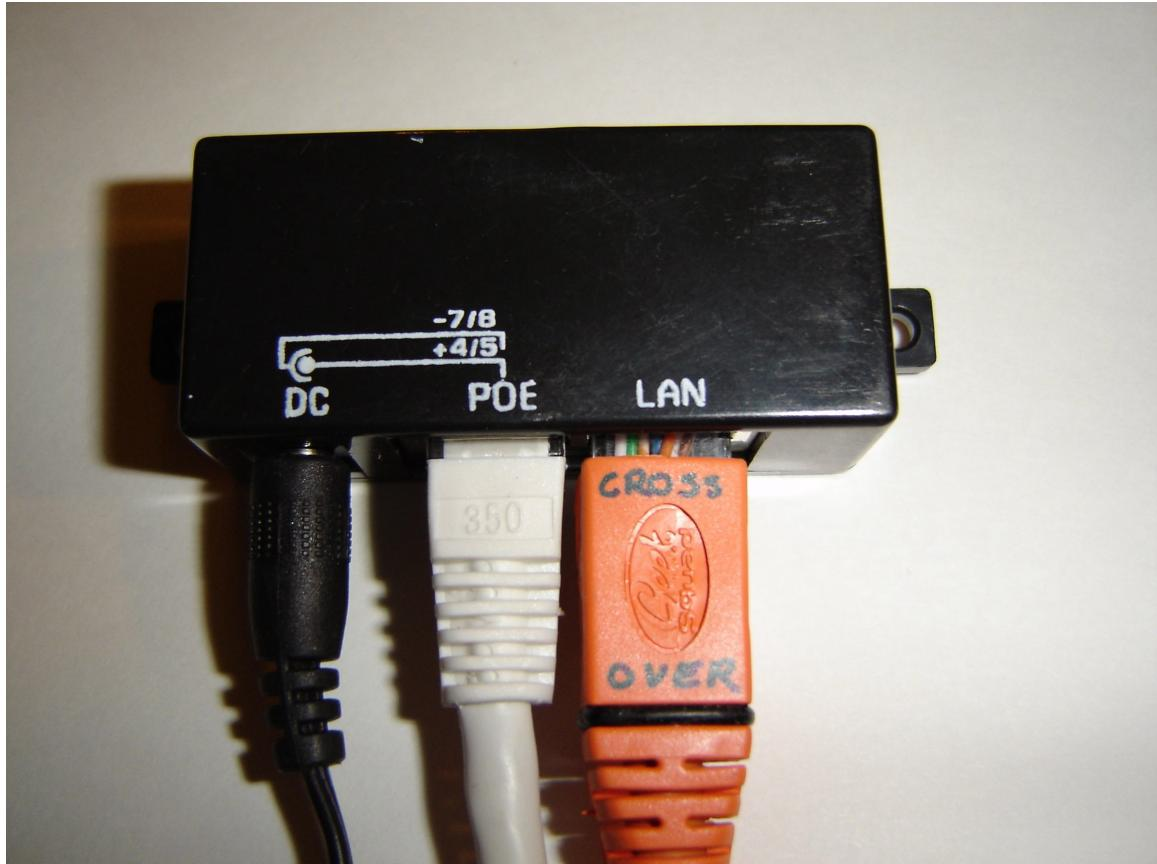
4. Plug the Ethernet cable into the Power over Ethernet Adapter (in the PoE port).
