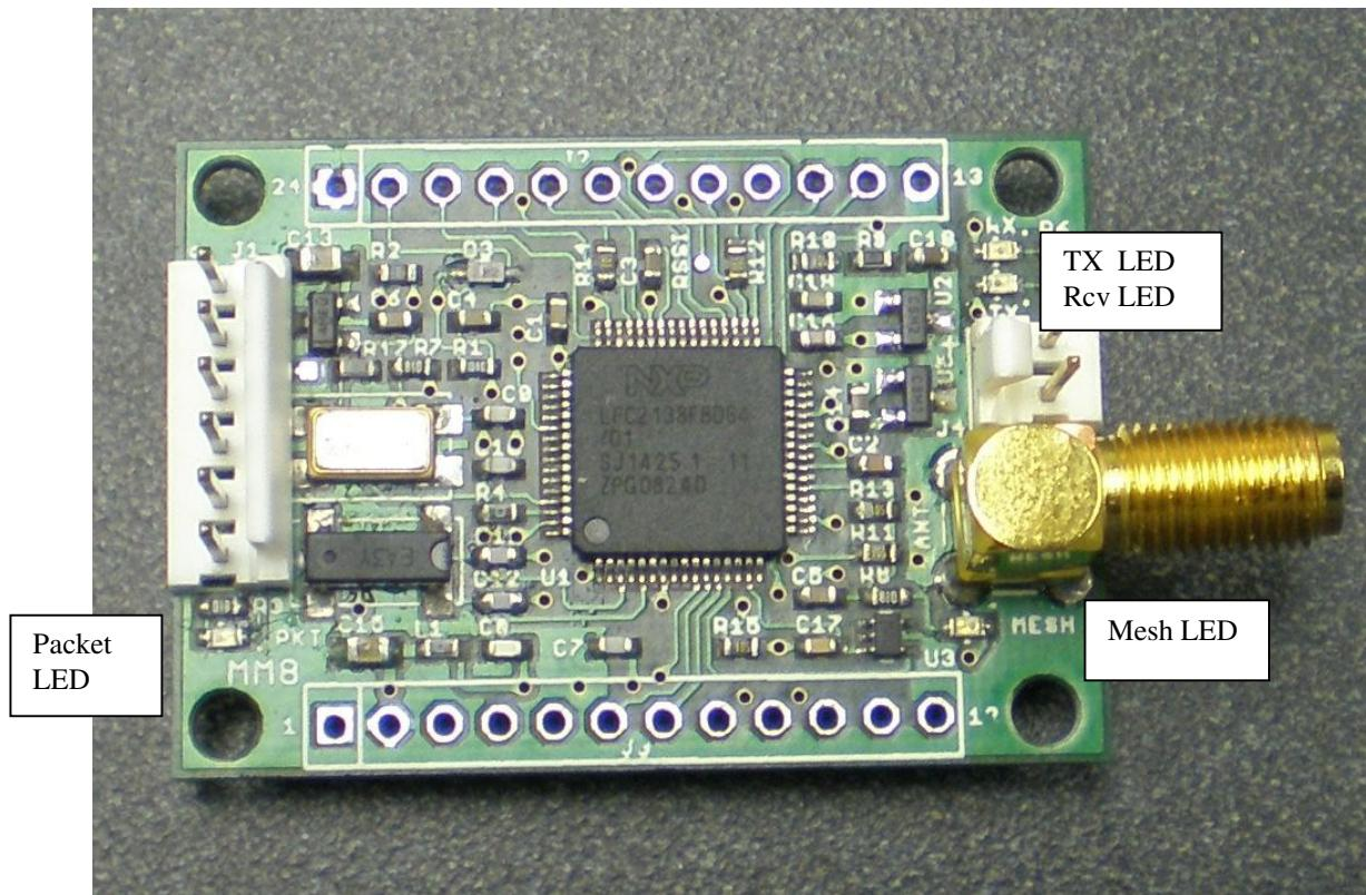
To assemble a MeshStamp® collect 3 alkaline AA batteries, one battery pack, one MeshStamp® antenna and one MeshStamp®. Then follow these steps for each of the MeshStamps®:
