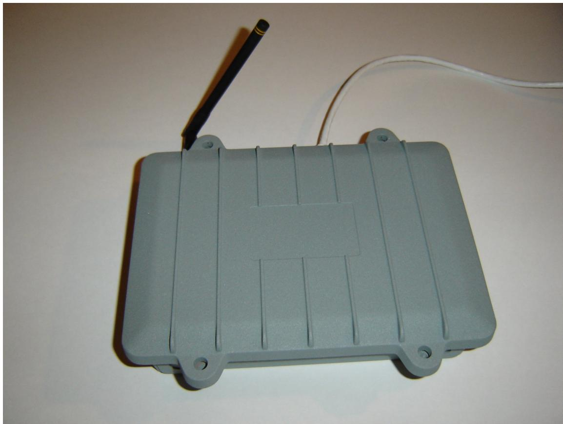
An Ethernet Gateway is powered through its Ethernet connector. A Power over Ethernet (PoE) adapter and its AC power cord is provided to power the Gateway.
