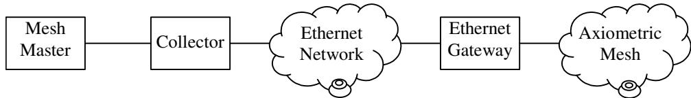
Mesh Master is an Axiometric developed JAVA based Network Manager application for MeshPlus® networks. It has two components, the first is the Mesh Master graphical user interface. The second is the Collector.
