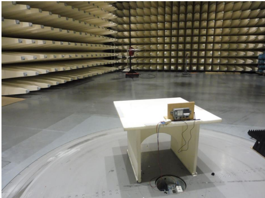
Photo 28: EUT at the semi-anechoic chamber with dipole antenna
