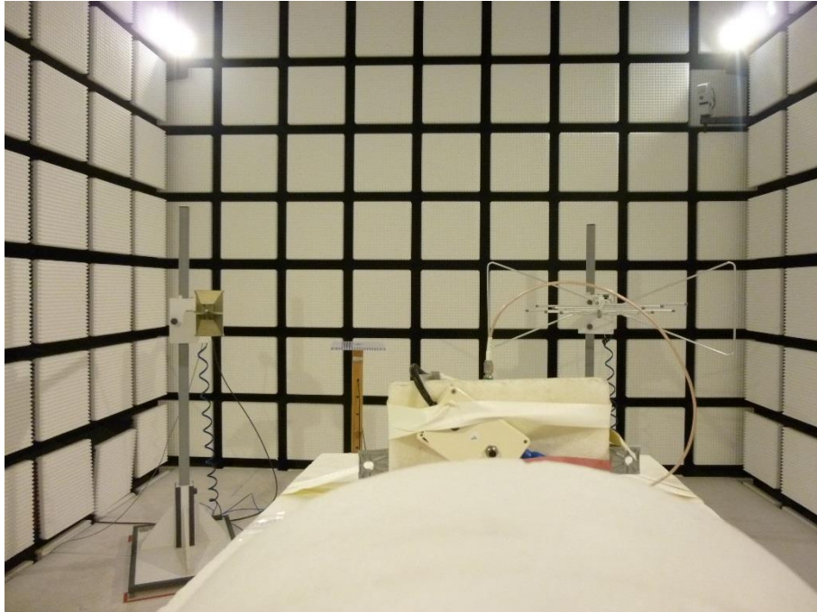
Photo 15: EUT at the anechoic chamber with spoiler antenna
