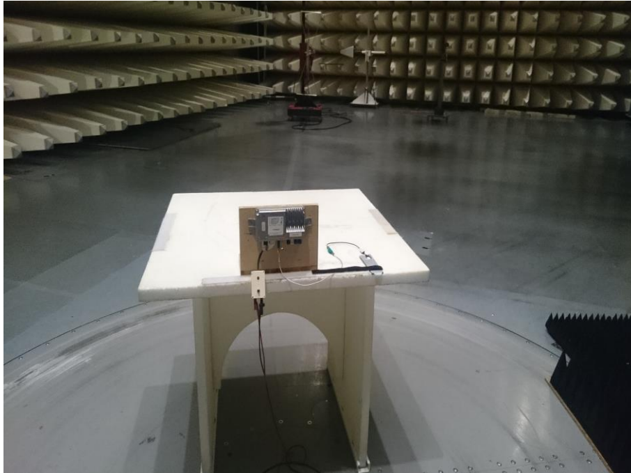
Photo 27: EUT at the semi-anechoic chamber with black print antenna
