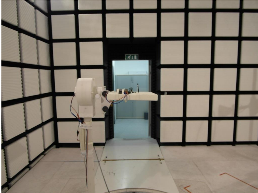
Photo 3: EUT at the anechoic chamber with dipole antenna
