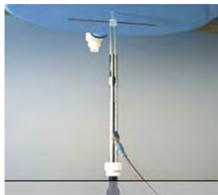
Photograph of the dipole Antenna
