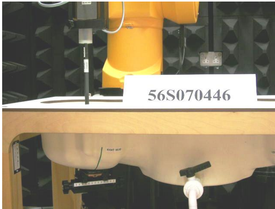
SAR Test Setup (Device at Head Phantom)
