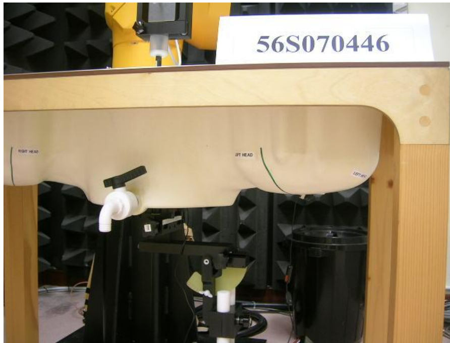
SAR Test Setup At Flat Phantom
