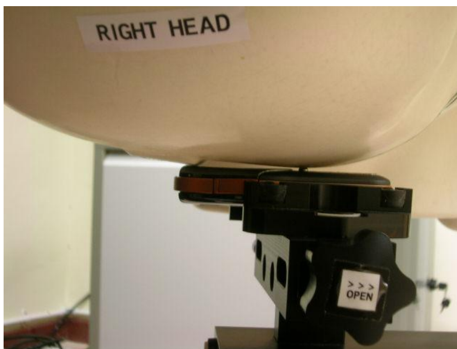
SAR Test Setup (Device at Head Phantom) – Closer Side View (Cheek/Touch)
