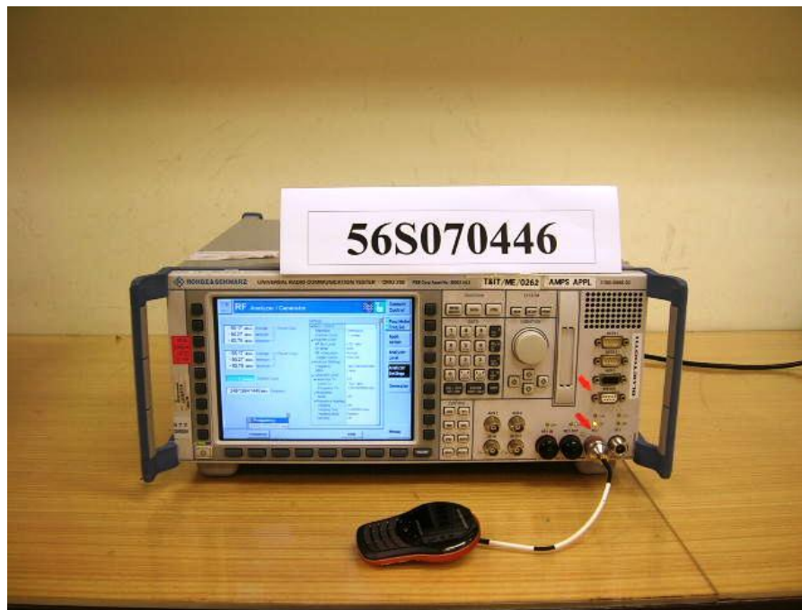
Conducted Power Measurement Setup
