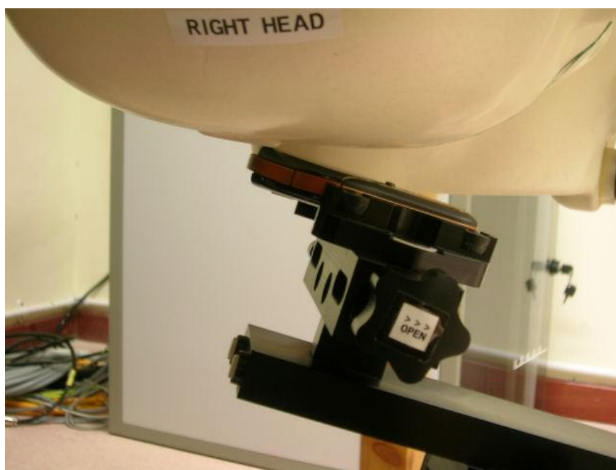
SAR Test Setup (Device at Head Phantom) – Closer Side View (Ear/Tilt)
