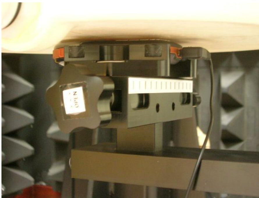
SAR Test Setup At Flat Phantom – Closer Front View (EUT Front Touched Phantom)
