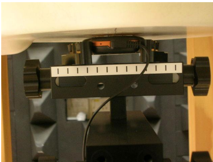
SAR Test Setup At Flat Phantom – Closer Side View (EUT Front Touched Phantom)
