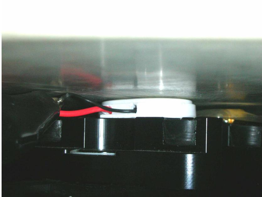
**SAR Test Setup Wrist Tag (Device at Flat phantom)**
