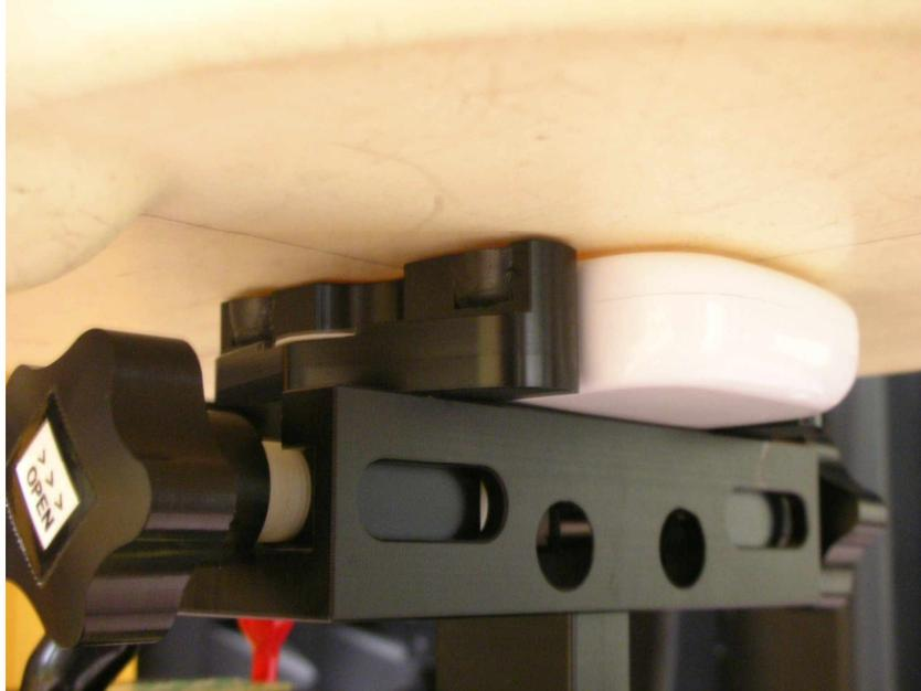
SAR Test Setup Base (Device at Flat phantom)
