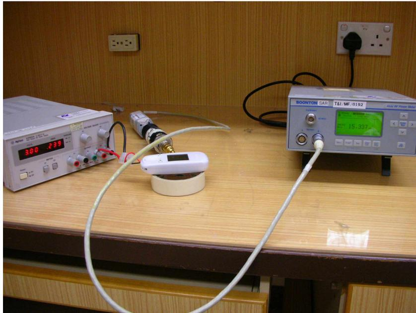
**Conducted power Test Setup Base**
