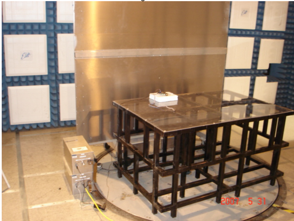
Test Set-up for Conducted Emissions
