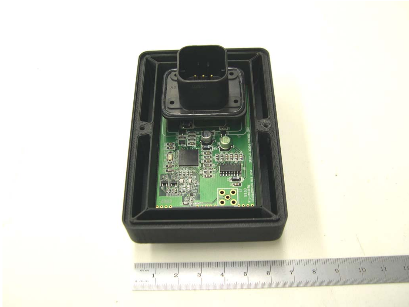
0G6019: PCB mounted in case.
