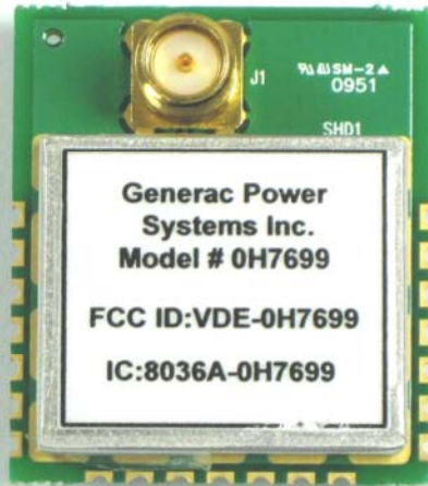
0H7699 module with connector for external antenna (see approved antennas listed below).
