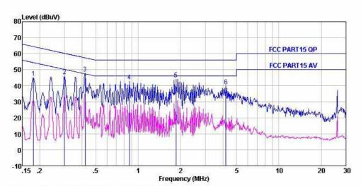
Condition: FCC PART15 QP LISN(2011) NEUTRAL EUT: Chumby NeTV Model: CHU-NTLV Test mode:: On mode Power: : AC 120V/60Hz Engineer:: David
