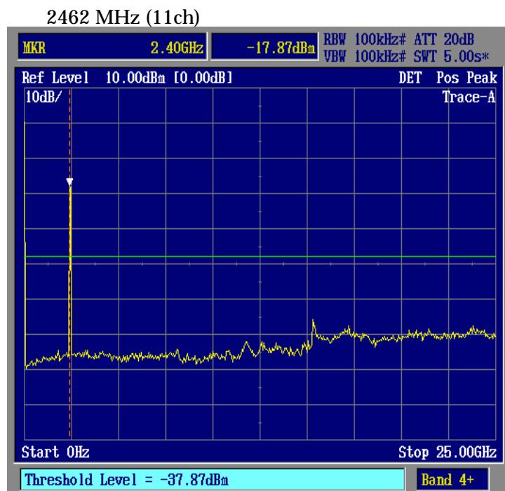
**5.5 15. 247(c) Transmitter Radiated Emissions (Radiated)****5.5.1 Setting Remarks**
