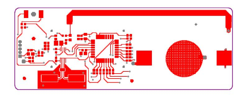
Printed circuit board antenna design
