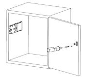
Step #6 - Screw the strike plate in place using 2 of the #6 x ½" screws supplied. If attaching to material less than 3/4" thick, alternate fasteners may be required.
