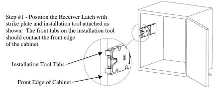
Step #2 - Screw the Receiver Latch in place using 4 of the #6 x ½" screws supplied. If attaching to material less than 3/4" thick, alternate fasteners may be required.
