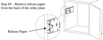
Step #5 – Close door firmly and open it again. The strike plate will become affixed to the door in the proper mounting position. Remove and discard red installation tool
