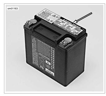
Figure 65. Battery Warning Label
