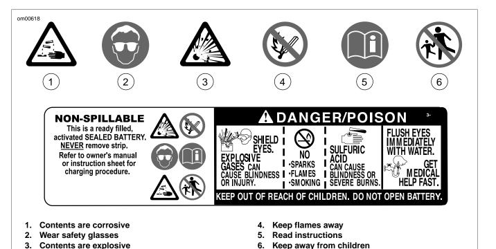
Figure 64. Battery Warning Label
