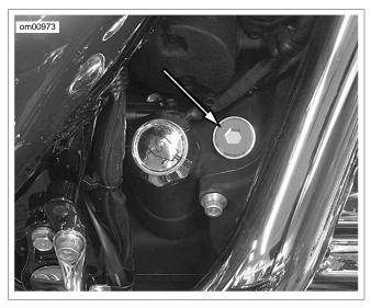
Figure 49. Transmission Filler Plug/Dipstick: FLHTCUSE3
