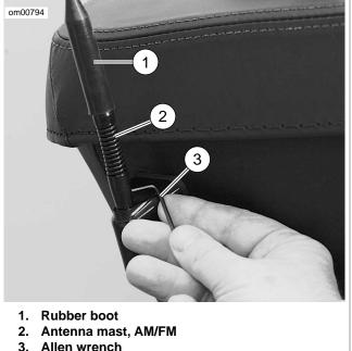
Figure 78. Radio Antenna: FLHTCUSE3
