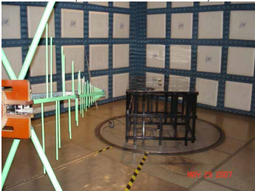
Test Setup for Radiated Emissions – Vertical Polarity
