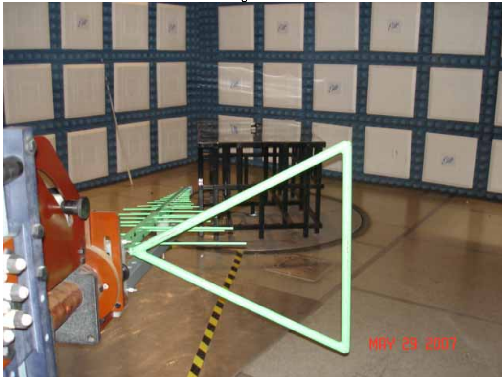
Test Setup for Radiated Emissions – Horizontal Polarity
