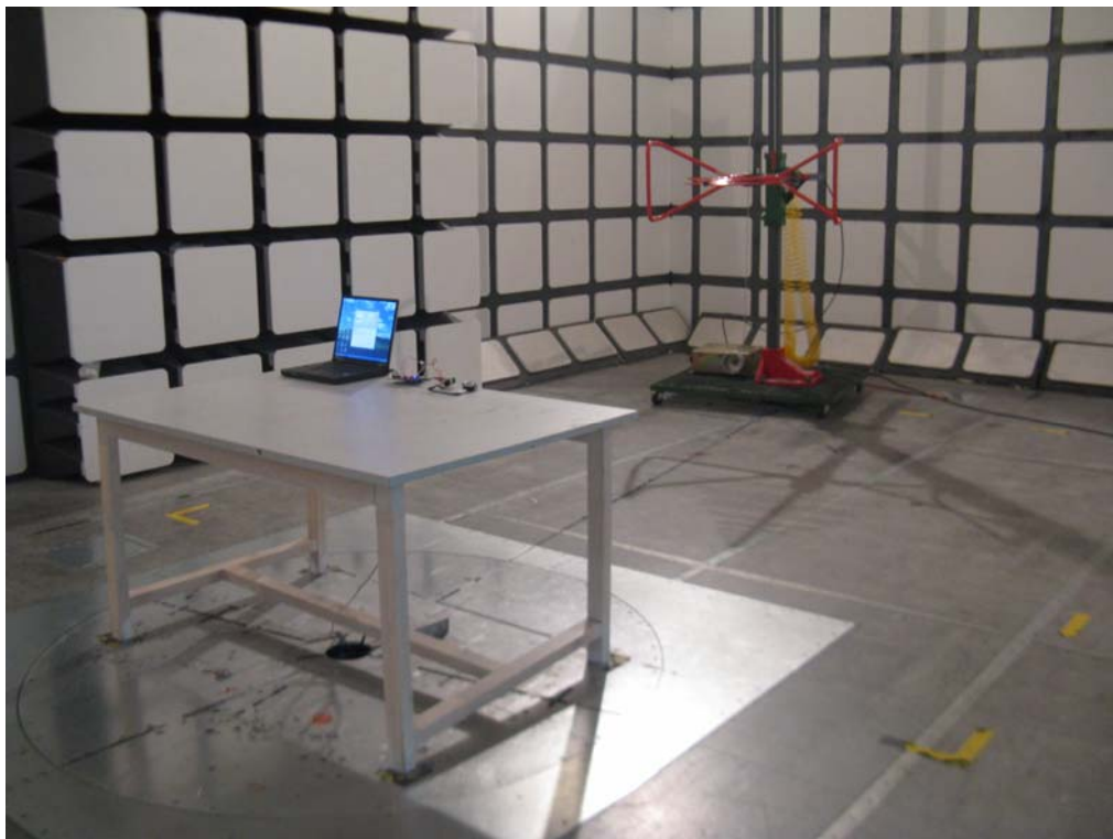
Transmitting mode: Radiated Emissions - Rear View (30 -1000 MHz)
