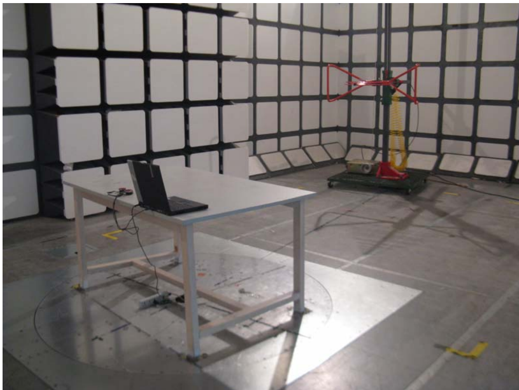
Charging mode: Radiated Emissions - Rear View (30 -1000 MHz)
