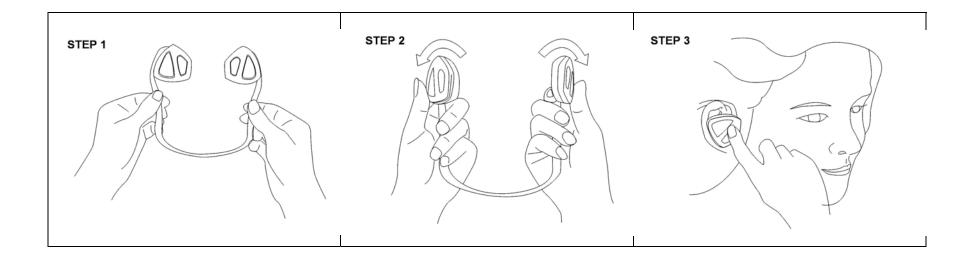
**NOTE**: Before attaching or detaching the ear-hook, first remove the ear cushion in case the ear cushion is broken.
