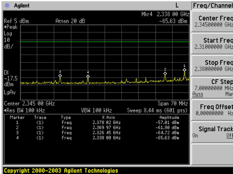
Conducted Emission Test Data CH-Mid
