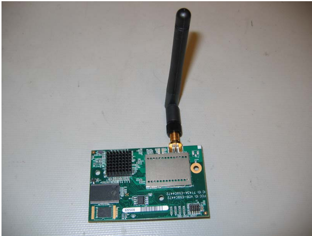
Figure 1 – RCM54XXW top view showing shield and antenna
