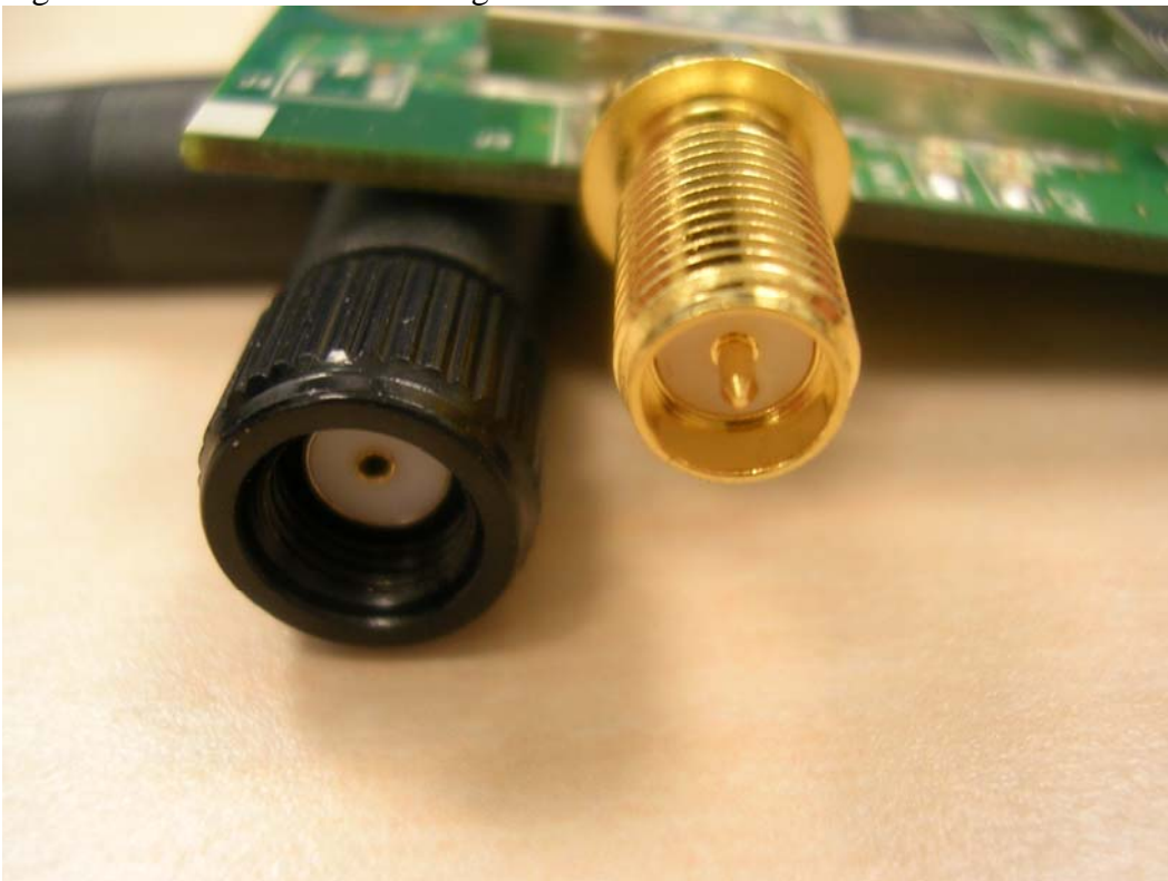
Figure 12. RCM4400W showing close-up of RP-SMA connector.
