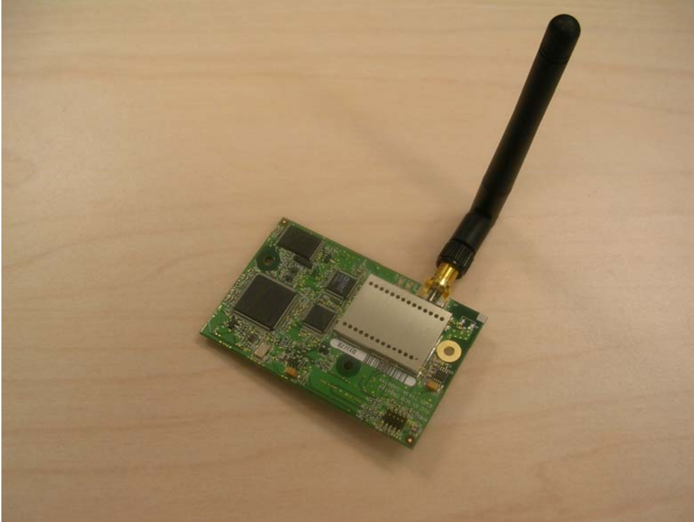
Figure 1. RCM4400W Showing RF shield and Omni-directional Antenna.
