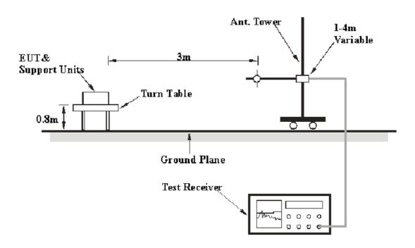
The radiated emission tests were performed in the chamber B test site, using the setup accordance with the ANSI C63.4-2003. The specification used was the FCC part 15.205, 15.209 and 15.235 limits.
