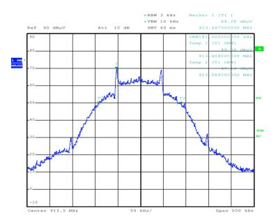
(913.5MHz - Middle) 99% bandwidth measured as 181kHz
