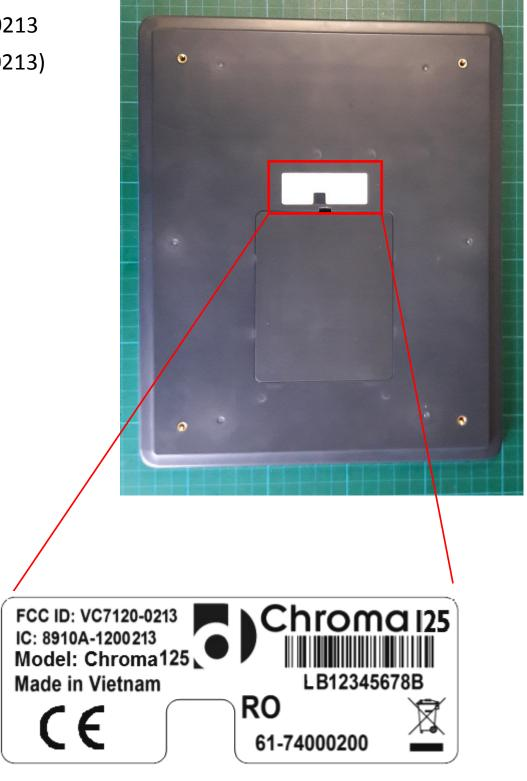
Label is placed on extenal face of rear cover, and is not removable.
