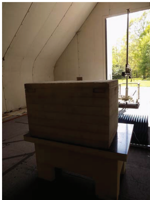
Radiated emissions, OATS, > 1000 MHz; 37L
