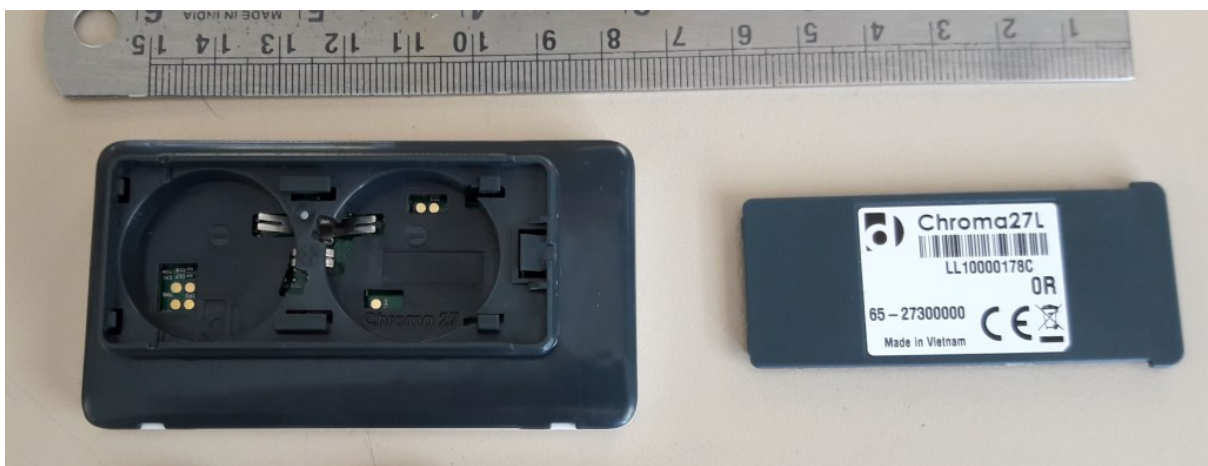
Battery Cover and 2 x CR2450 coin cells removed
