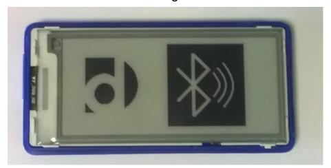
Front view with display folded back – showing display support.
