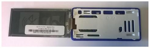
Front view with display folded back and support removed – showing PCB and antennas
