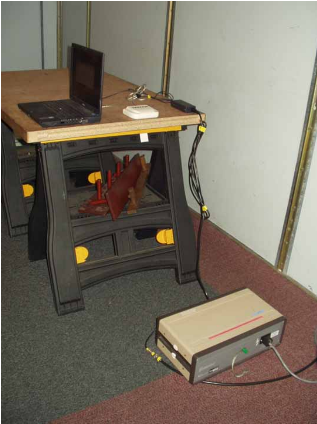
Photograph of the EUT as viewed from screened room (conducted emissions)
