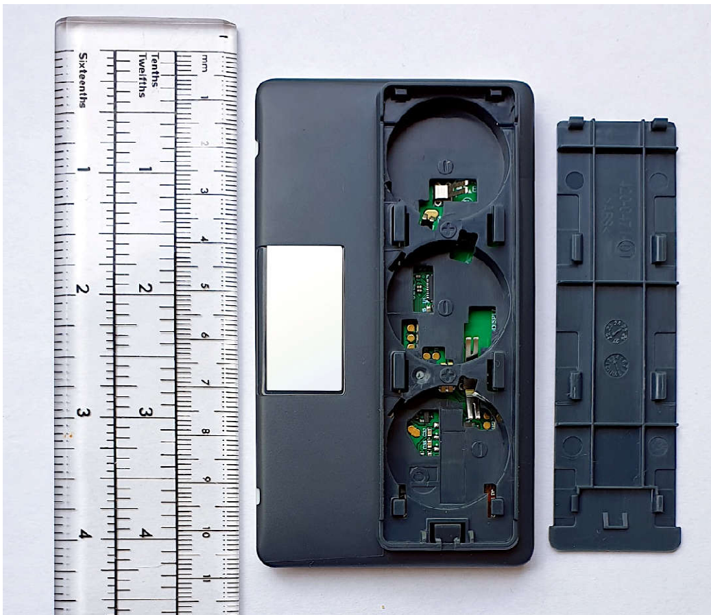
DD37-3A (Chroma 37L) – Front Cover, Battery Cover and Coin cell removed.
