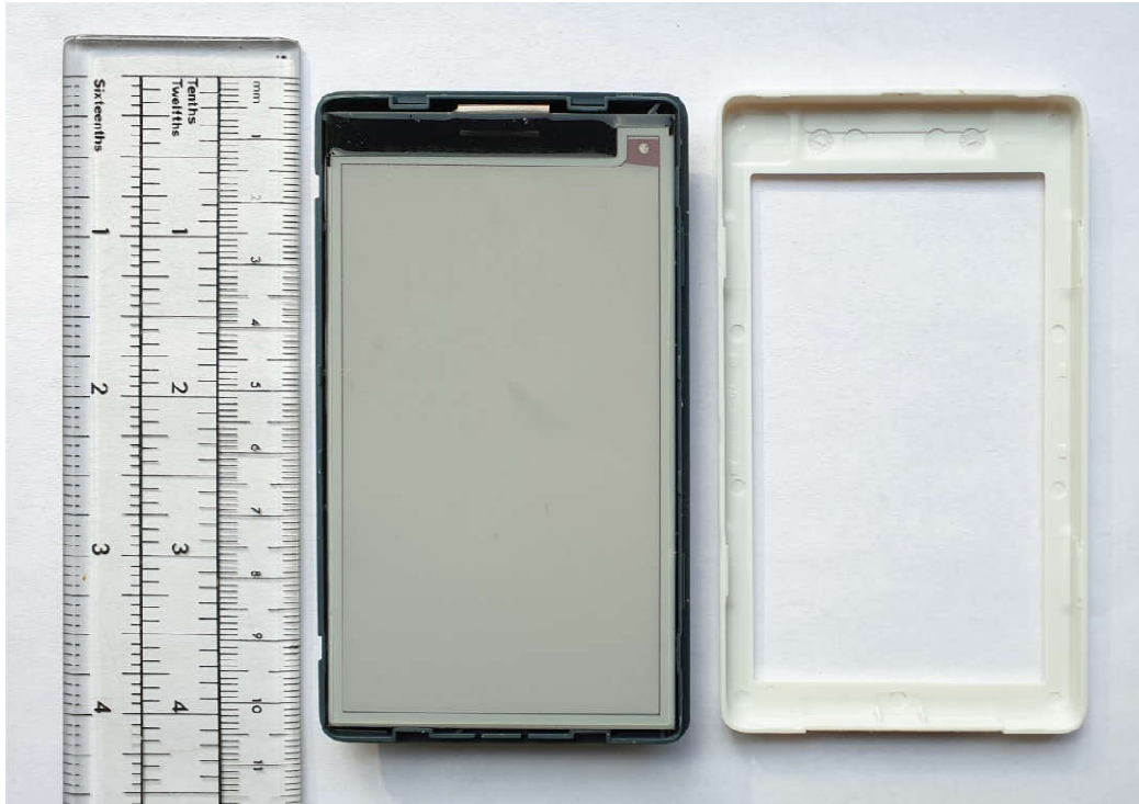
DD37-3A (Chroma 37+) – Front Cover, Battery Cover and Coin cell removed.
