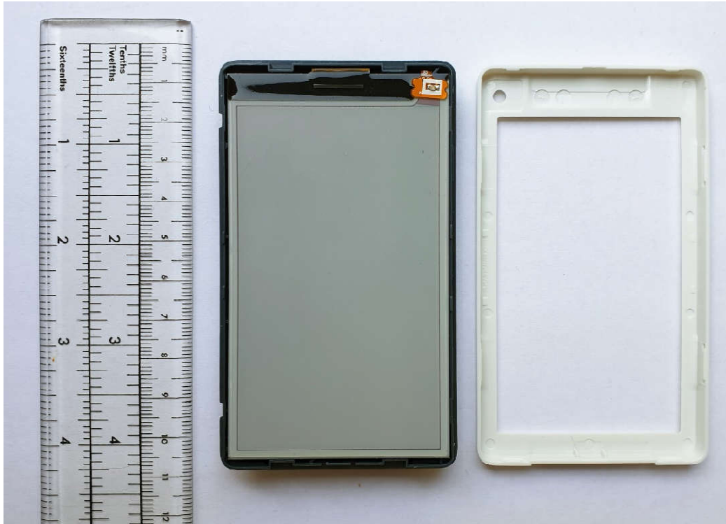
DD37-3A (Chroma 37L) – Battery Cover and Coin cell removed.
