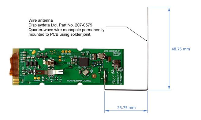
Note, all measurements in the associated Test Report exhibit for Model Number / HVIN: DD37-3A, are radiated measurements, therefore additional antenna gain documentation is not required.
