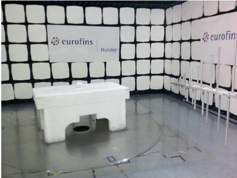
Radiated Emissions; Above 1GHz
