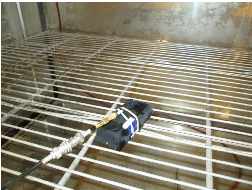
Photo 4.6.2 Test setup regarding measurement of carrier frequency stability. Test object in climate chamber.
